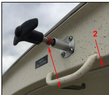
Latched (2) but unlocked (1) WRONG!
