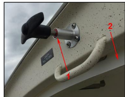
Clearly locked (1) but unlatched (2) WRONG!
