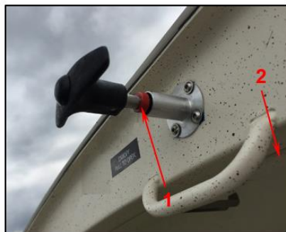
Latched (2) but partially locked (1) WRONG!
